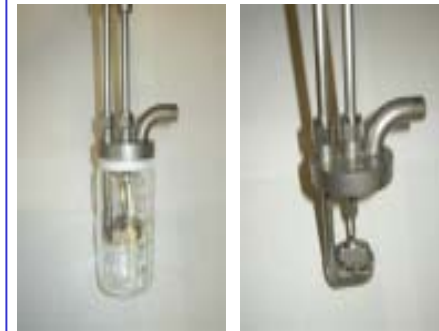
Figure 1. Left picture shows the assembled "bubbling" aerosol generator while the right panel shows the porous disk and liquid delivery system. Drying air may be added tangentially if needed.
